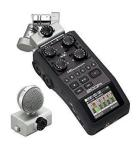
6 Input, 6-Track Portable Recorder with Interchangeable Mic Capsules, .WAV .MP3, 96Khz 48+44.1Khz, 16-bit Charger, 16GB USB Card, Windscreen, USB2
